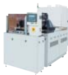
Multi-layer single substrate sputtering equipment
